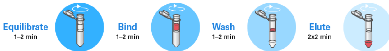
Figure 1. Rapid miniprep workflow for EV purification. With the Capturem Extracellular Vesicle Isolation Kit (Mini), EVs are first bound to the equilibrated membrane, and then washed and eluted with the appropriate buffers. Each step is followed by spinning the tube for just 1–2 minutes at 500g.
