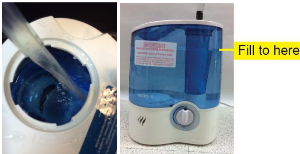
Figure 15. Filling the Reservoir with deionized water.
