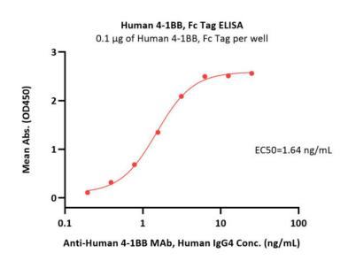
Immobilized Human 4-1BB, Fc Tag (Cat. No. 41B-H5258) at 1  $\mu$ g/mL (100  $\mu$ L/well) can bind Anti-Human 4-1BB MAb, Human IgG4 with a linear range of 0.2-3 ng/mL (Routinely tested).
