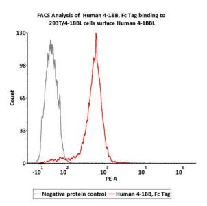
Flow Cytometry assay shows that Human 4-1BB, Fc Tag (Cat. No. 41B-H5258) can bind to 293T cells overexpressing Human 4-1BBL. The concentration of 4-1BB used is 0.1 µg/mL (Routinely tested).
