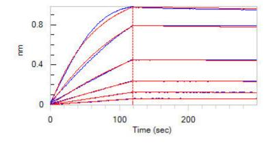
Loaded Human 4-1BB, Fc Tag (Cat. No. 41B-H5258) on Protein A Biosensor, can bind Human 4-1BB Ligand, His Tag with an affinity constant of 1.3 nM as determined in BLI assay (ForteBio Octet Red96e) (Routinely tested).
