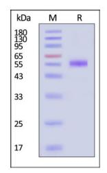
Human 4-1BB, Fc Tag on SDS-PAGE under reducing (R) condition. The gel was stained with Coomassie Blue. The purity of the protein is greater than 90% (With <u>Star Ribbon Pre-stained Protein Marker</u>).
