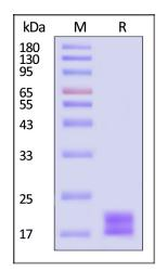
Human PD-L1 (19-134), His Tag on SDS-PAGE under reducing (R) condition. The gel was stained with Coomassie Blue. The purity of the protein is greater than 95% (With <u>Star Ribbon Pre-stained Protein Marker</u>).
