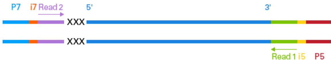
Figure 2. Structural features of final libraries generated with the SMARTer Stranded Total RNA-Seq Kit v2 - Pico Input Mammalian. The adapters added using 5' PCR Primer HT and 3' PCR Primer HT contain sequences allowing clustering on any Illumina flow cell (P7 shown in light blue, P5 shown in red), Illumina TruSeq® HT indexes (Index 1 [i5] sequence shown in yellow, and Index 2 [i7] sequence shown in orange), as well as the regions recognized by sequencing primers Read Primer 2 (Read 2, purple) and Read Primer 1 (Read 1, green). Read 1 generates sequences antisense to the original RNA, while Read 2 yields sequences sense to the original RNA (orientation of original RNA denoted by 5' and 3' in dark blue). The first three nucleotides of the second sequencing read (Read 2) are derived from the Pico v2 SMART Adapter (shown as Xs). These three nucleotides must be trimmed prior to mapping if performing paired-end sequencing.
